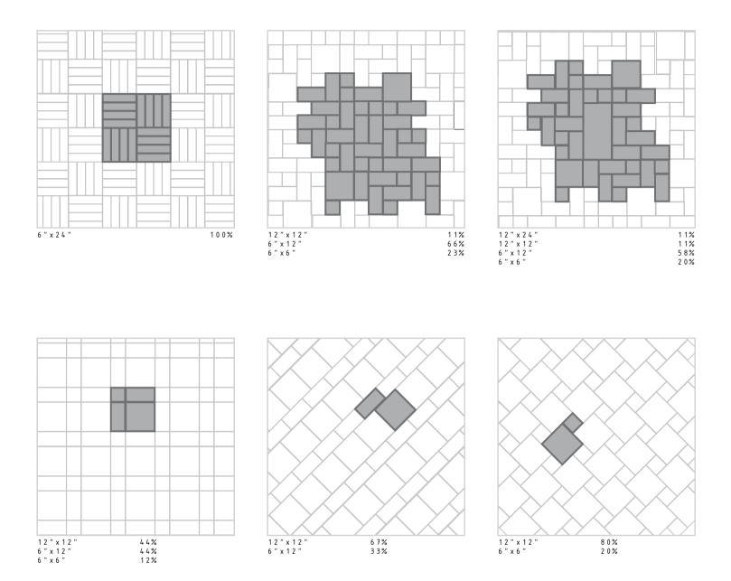
MODULARITY WILL DIFFER BASED ON WHETHER THE PRODUCT IS RECTIFIED OR CALIBRATED Color-lined pieces indicate the pattern. Calculations have been rounded to the nearest percentage. It is recommended to round "up" when calculating square footage.
