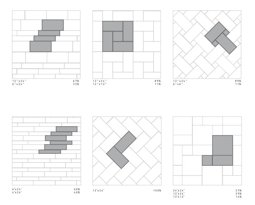
MODULARITY WILL DIFFER BASED ON WHETHER THE PRODUCT IS RECTIFIED OR CALIBRATED Color-lined pieces indicate the pattern. Calculations have been rounded to the nearest percentage. It is recommended to round "up" when calculating square footage.
