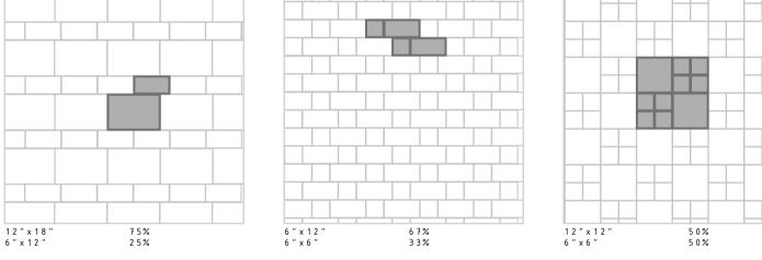
MODULARITY WILL DIFFER BASED ON WHETHER THE PRODUCT IS RECTIFIED OR CALIBRATED
